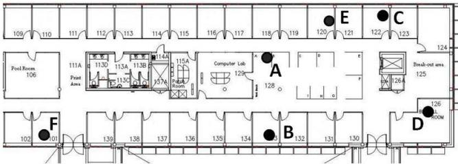
Fig. 1. Floorplan of our office with measurement locations (95m  $\times$  18m). The area left of A is an open floor office area. Above and below are regular offices. Most of the obstacles are glass, wood or concrete. The only exception is the elevator, lying in between C and D, which has a thick concrete and metal case.
