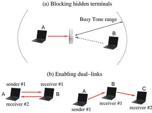
**Figure 1: (a) Handling hidden terminals:** The transmission from  $A$  to the access point is protected from the hidden node  $B$  by the busy tone/packet sent by the access point while receiving the packet from  $A$ . **(b) Enabling dual links:** using self-interference cancellation at nodes  $A$  and  $B$ , we can activate two links simultaneously, i.e., dual links - (left) a symmetric dual link ( $A, B, A$ ), (left) an asymmetric dual link ( $A, B, C$ ).
