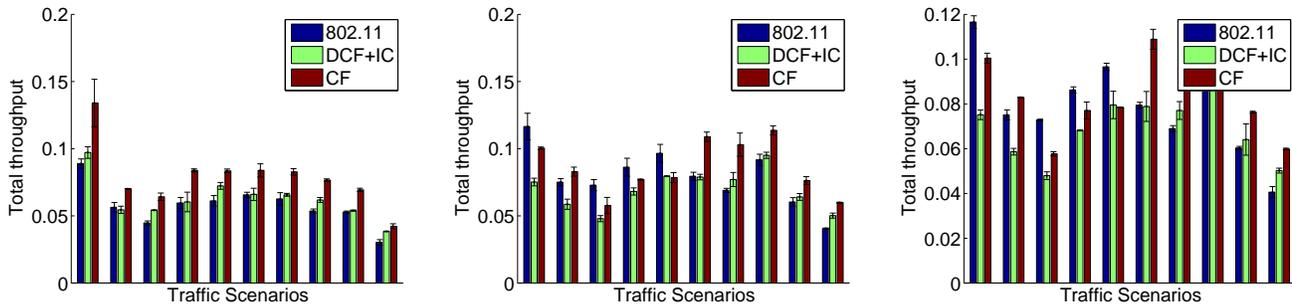
Figure 12: Total throughput of network topologies 1 (left), 2 (middle) and 3 (right). X axis denotes different traffic matrices and Y axis is the total throughput.
