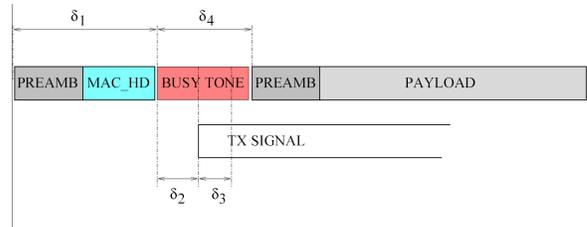
Figure 8: A structure of a packet transmitted on a dual link. The figure depicts a secondary transmitter receiving a packet, and starting a secondary transmission in the case of indirect cancellation.
