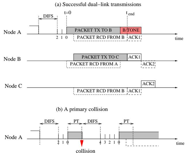
**Figure 6: (a) An example of successful transmissions on an asymmetric dual-link. (b) A primary collision experienced by node  $A$ .**
